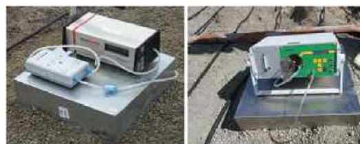
Fig. 2. The two monitors used: on the left AlphaGUARD PQ2000 and on the right the EQF 3120.
