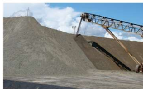
Fig. 1. The crushed uranium ore pile formation.
