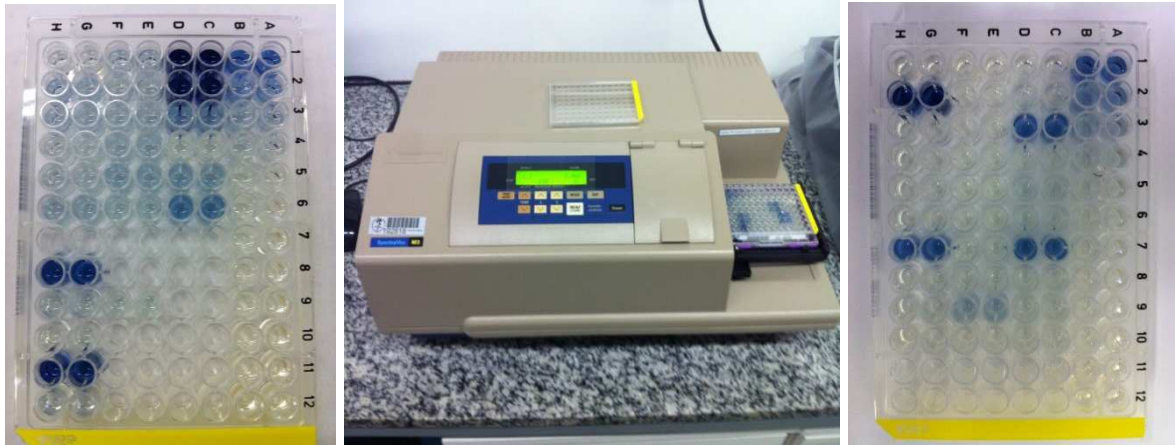
Fig. 3.6: SpectraMax M3 Multimode Reader (Molecular Devices Inc.) used in a biochemical determinations of ALP concentrations in 96 plate wells by reading the absorbance at 630 nm. The columns A and B of the 96 plate wells were filled with the standard curve (1 to 9) and blank samples (10 to 12). The columns C to H (1 to 12) was filled in duplicate (C-D; E-F; G-H) with samples.
