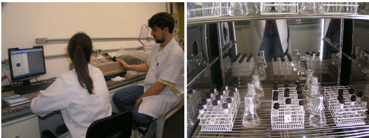
Fig. 3.11: Algae inhibition growth test in D. subspicatus and P. subcapitata (single and combined) exposed to hormones spiked water for 96 h. Vials randomly arranged in racks.
