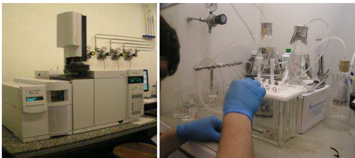
Fig. 3.13: GC-MS Gas Chromatography (7890A Agilent) coupled to mass spectrometry (5975C triplo axis detector). Solid phase extraction (SPE) in an Agilent Bond Elut C-18, 500 mg, 3 ml cartridges.
